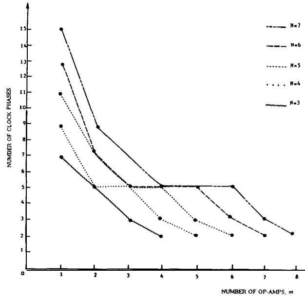
Fig. 3. Multiplexed Nth-order filter with  $m$  op-amps.
