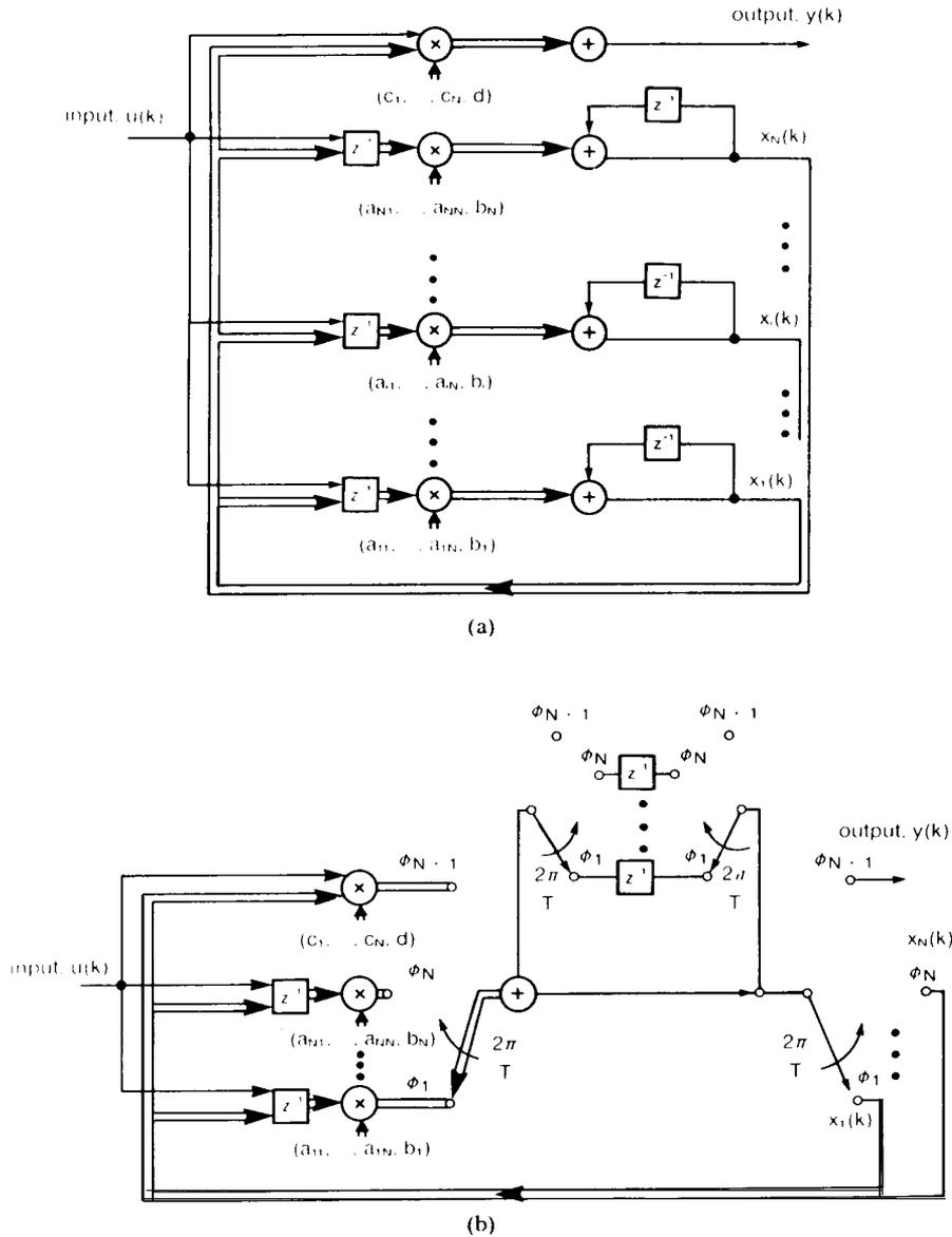
Fig. 1. Functional representation of A domain state-space structure in (a) nonmultiplexed form and (b) multiplexed form.
