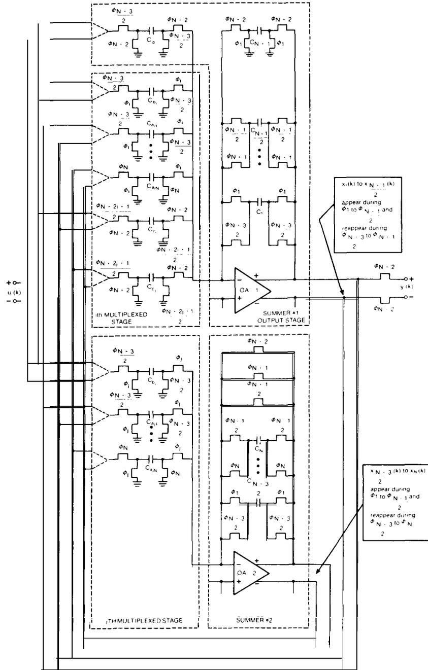
Fig. 4. Multiplexed SC circuit with two op-amps,  $N$  odd (only one-half the fully differential circuit is shown),
